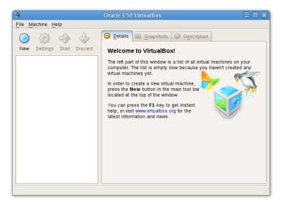
On the left, you can see a pane that will later list all your virtual machines. Since you have not created any, the list is empty. A row of buttons above it allows you to create new VMs and work on existing VMs, once you have some. The pane on the right displays the properties of the virtual machine currently selected, if any. Again, since you don't have any machines yet, the pane displays a welcome message.
