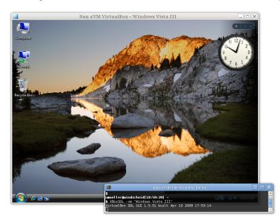
To start a virtual machine with VBoxSDL instead of the VirtualBox GUI, enter the following on a command line:
