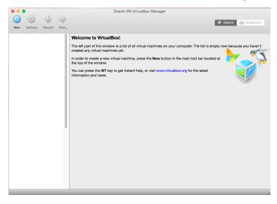
This window is called the "VirtualBox Manager". On the left, you can see a pane that will later list all your virtual machines. Since you have not created any, the list is empty. A row of buttons above it allows you to create new VMs and work on existing VMs, once you have some. The pane on the right displays the properties of the virtual machine currently selected, if any. Again, since you don't have any machines yet, the pane displays a welcome message.
