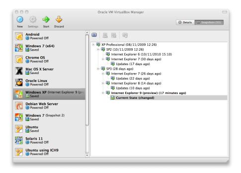
VirtualBox imposes no limits on the number of snapshots you can take. The only practical limitation is disk space on your host. Each snapshot stores the state of the virtual machine and thus occupies some disk space. See chapter 1.11.2, *Snapshot Contents*, page 30 for details on what is stored in a snapshot.
