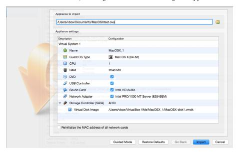
This presents the virtual machines described in the OVF file and allows you to change the virtual machine settings by double-clicking on the description items. Once you click on "Import", VirtualBox will copy the disk images and create local virtual machines with the settings described in the dialog. These will then show up in the Manager's list of virtual machines.
