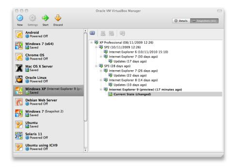
VirtualBox imposes no limits on the number of snapshots you can take. The only practical limitation is disk space on your host: each snapshot stores the state of the virtual machine and thus occupies some disk space. (See the next section for details on what exactly is stored in a snapshot.)
