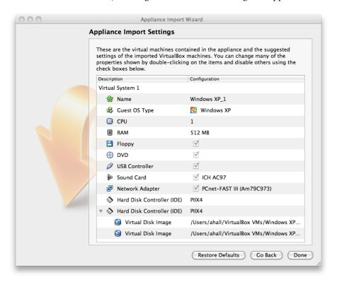
This presents the virtual machines described in the OVF file and allows you to change the virtual machine settings by double-clicking on the description items. Once you click on "Import", VirtualBox will copy the disk images and create local virtual machines with the settings described in the dialog. These will then show up in the Manager's list of virtual machines.
