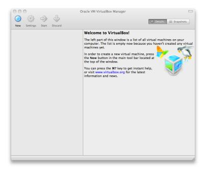
This window is called the "VirtualBox Manager". On the left, you can see a pane that will later list all your virtual machines. Since you have not created any, the list is empty. A row of buttons above it allows you to create new VMs and work on existing VMs, once you have some. The pane on the right displays the properties of the virtual machine currently selected, if any. Again, since you don't have any machines yet, the pane displays a welcome message.
