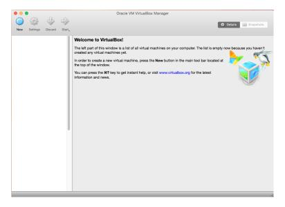
This window is called the "VirtualBox Manager". On the left, you can see a pane that will later list all your virtual machines. Since you have not created any, the list is empty. A row of buttons above it allows you to create new VMs and work on existing VMs, once you have some. The pane on the right displays the properties of the virtual machine currently selected, if any. Again, since you do not have any machines yet, the pane displays a welcome message.
