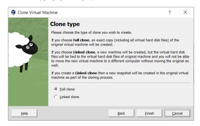
The **Clone Type** option specifies whether to create a clone that is linked to the source VM or to create a fully independent clone:
