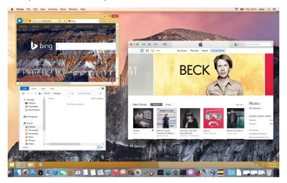
To enable seamless mode, after starting the virtual machine, press the **Host key + L**. The Host key is normally the right control key. This will enlarge the size of the VM's display to the size of your host screen and mask out the guest operating system's background. To disable seamless windows and go back to the normal VM display, press the Host key + L again.
