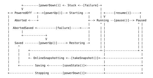
Note that states to the right of PoweredOff, Aborted, AbortedSaved, and Saved in the above diagram are called *online VM states*. These states represent the virtual machine which is being executed in a dedicated process (usually with a GUI window attached to it where you can see
